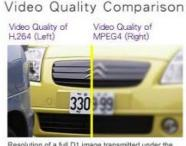
Resolution of a full D1 image transmitted under the same bandwidth condition when adopting a different technology.
