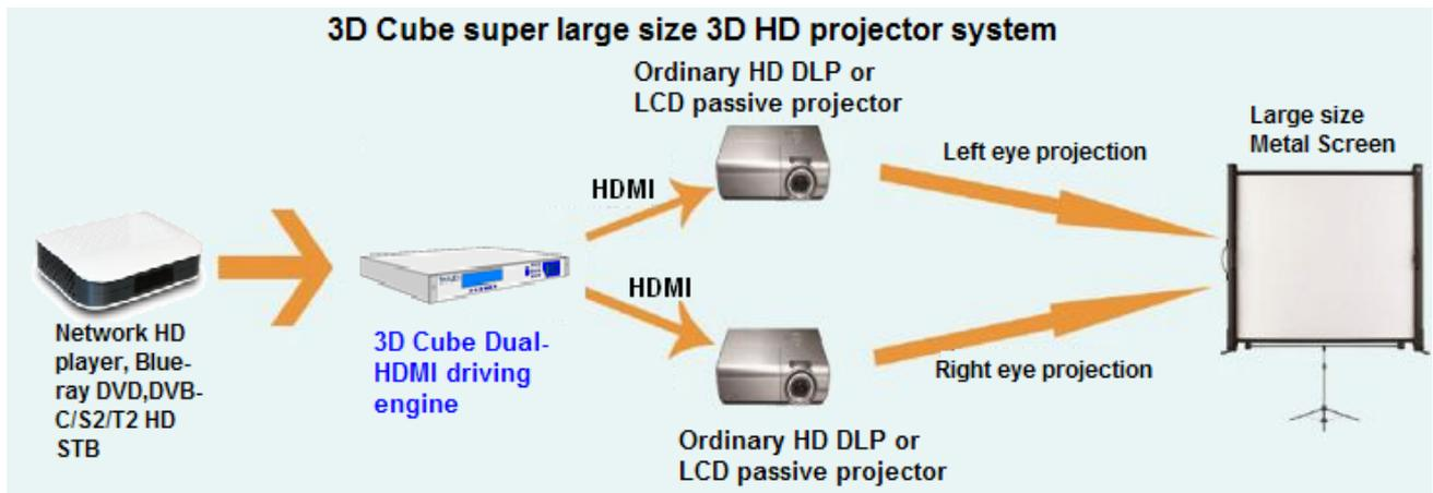
So, one super large size 3D HD projector system is composed of 3D Cube Dual-HDMI driving engine as the center, two ordinary and economic HD 1080P/i 2D DLP or LCD passive projectors with same type, two circular or linear polarization lens (corresponding to DLP or LCD passive projector), and one large size metal screen.
